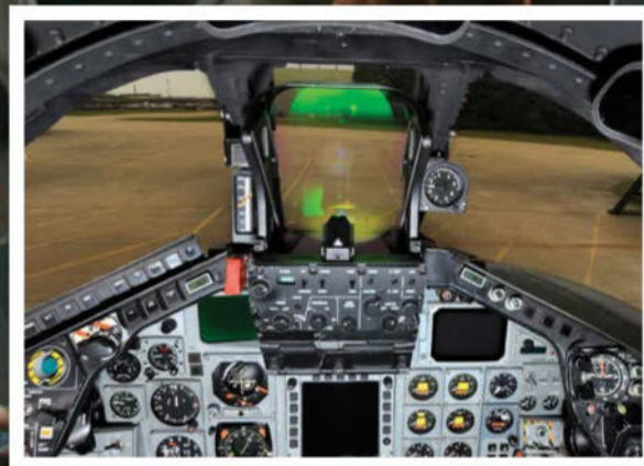
Right: The pilot looked through a Head-Up Display (HUD)
